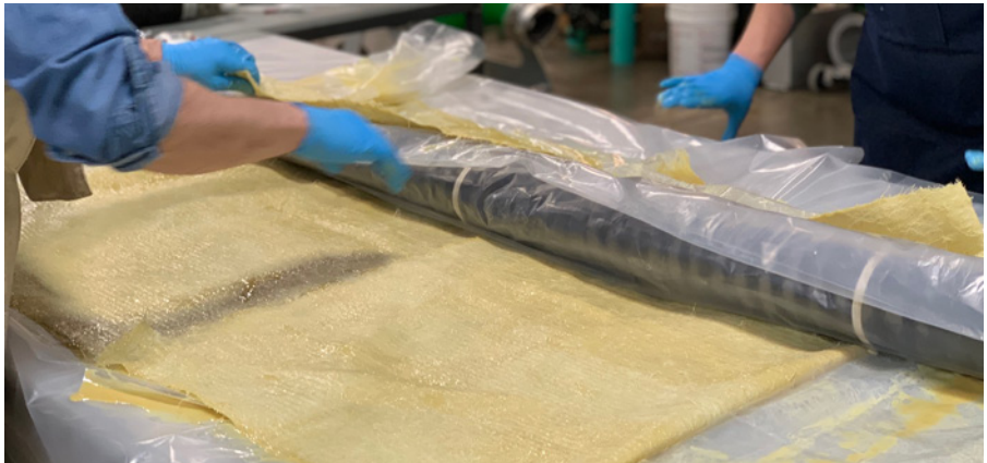
Fig. 8 Place the polythene-covered lateral packer on the mat so that the mat sits between the reference lines.
