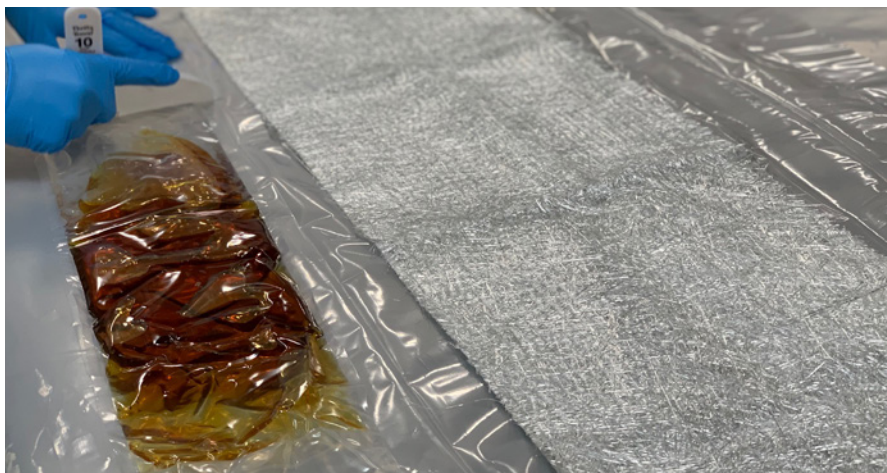
Fig. 5 Activate your resin pack and massage it from the outside for at least one minute to ensure that it is fully mixed.
