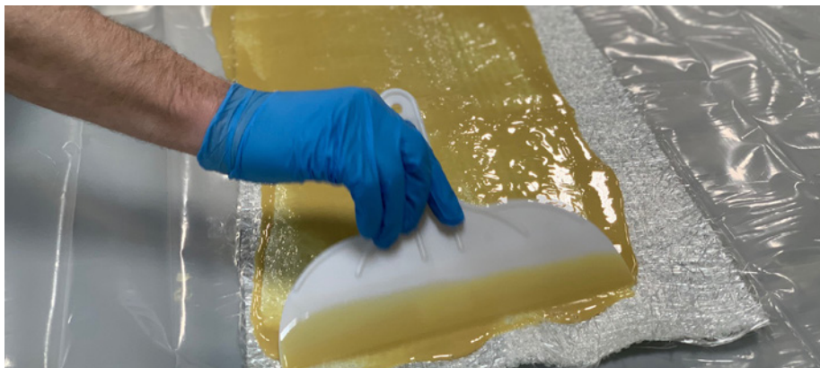
Fig. 6 Pour the well-mixed resin onto the fibreglass matting and spread out evenly.
