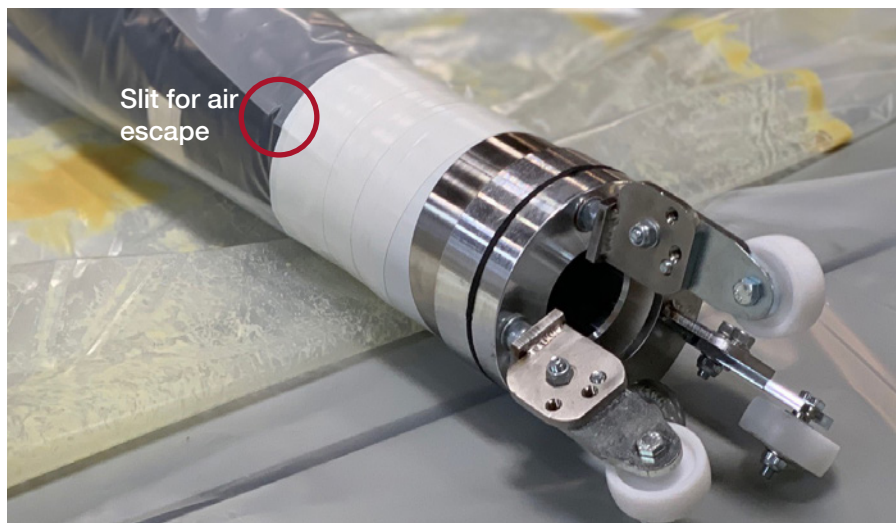
Fig. 4 Placing tape around the ends of the flexible packer.
