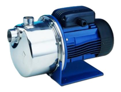
Our inlet water pumps are close-coupled self-priming centrifugal pumps with built-in ejector systems, designed to remain primed even in the presence of water-dissolved gases.
