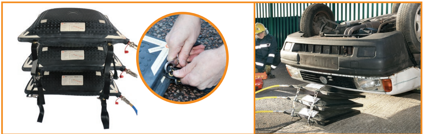
Fig 5.20: Combining Stak Jaks to increase lifting height
